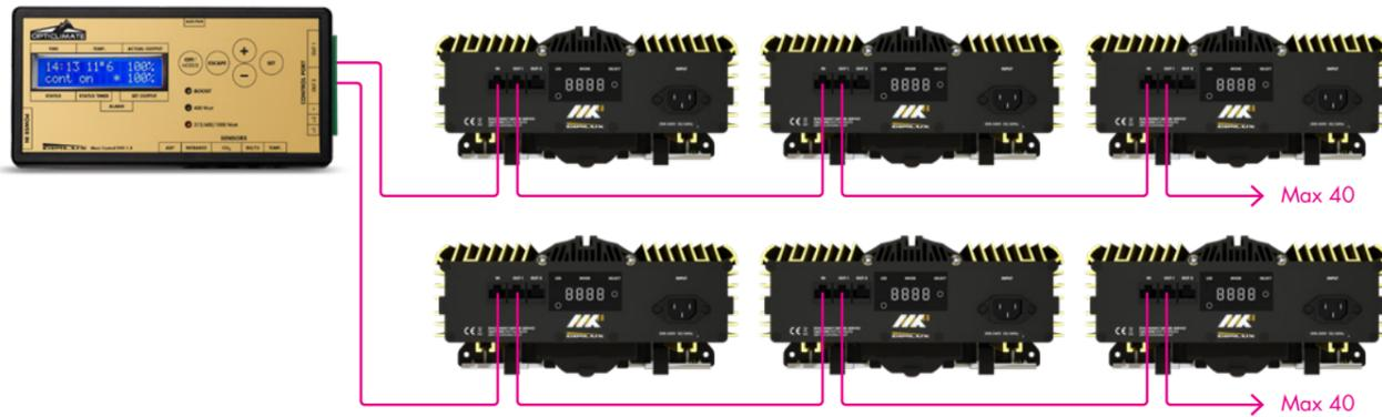
For more than 80 fixtures, use a splitter and divide equally between OUT-1 and OUT-2
