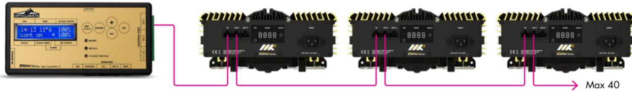
For more than 20 fixtures, it is recommended to divide equally between ports OUT-1 and OUT-2 (up to 80 fixtures)
