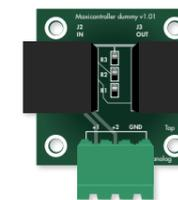
If you want to keep your old controller or use a different control system you can use the Maxi Controller Dummy Adapter which must be placed between the old Maxi Controller and the first ballast or fixture.
